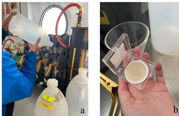
**Fig. 5.13** a) Filtration in the laboratory b) Glass fiber filter after filtration
