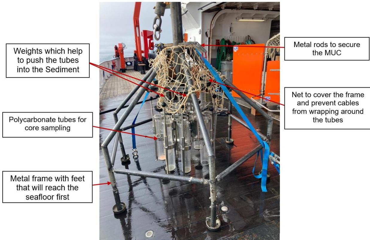
**Fig. 5.19** The multicorer with a description of the components.
