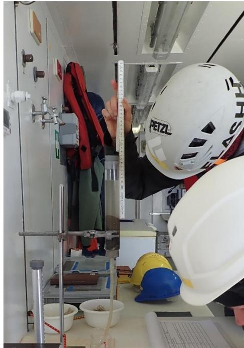
**Fig. 5.17** Measuring the water level in the glass tube.
