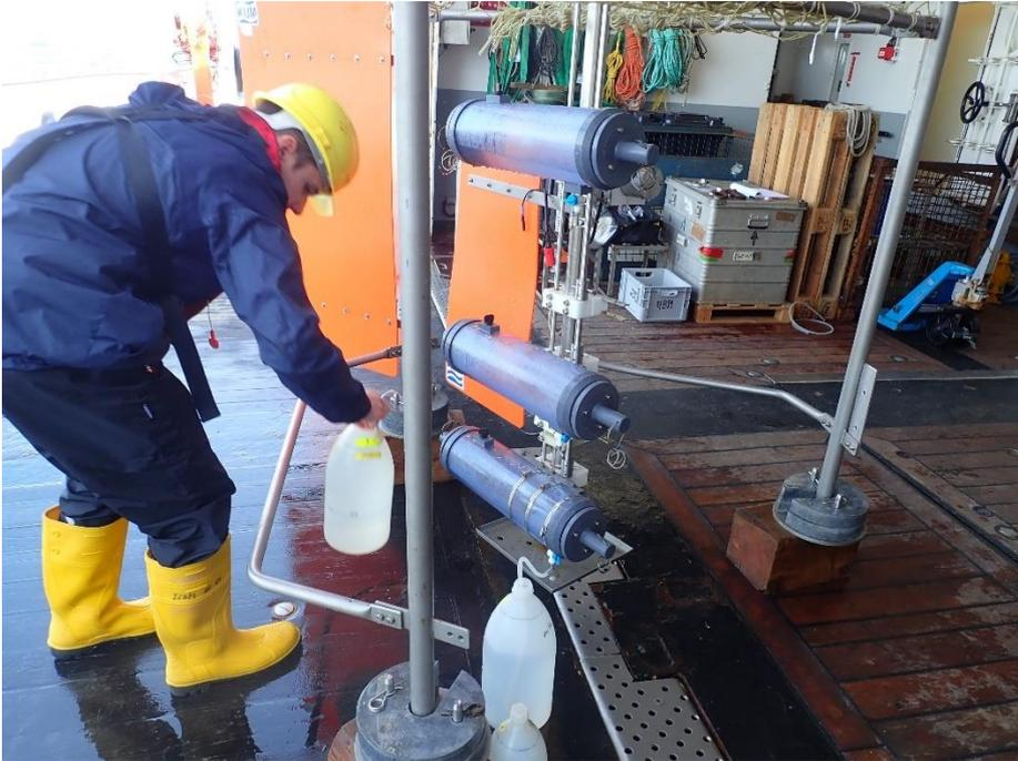
**Fig. 11.9** Filling bottles with the BWS samples.
