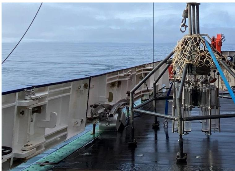
**Fig. 5.16** The van Veen grab on deck, with the multicorer to the right.
