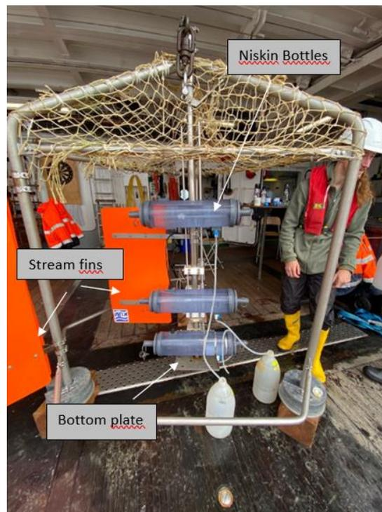
**Fig. 5.11** The Bottom Water Sampler (BWS) used during cruise HE639.
