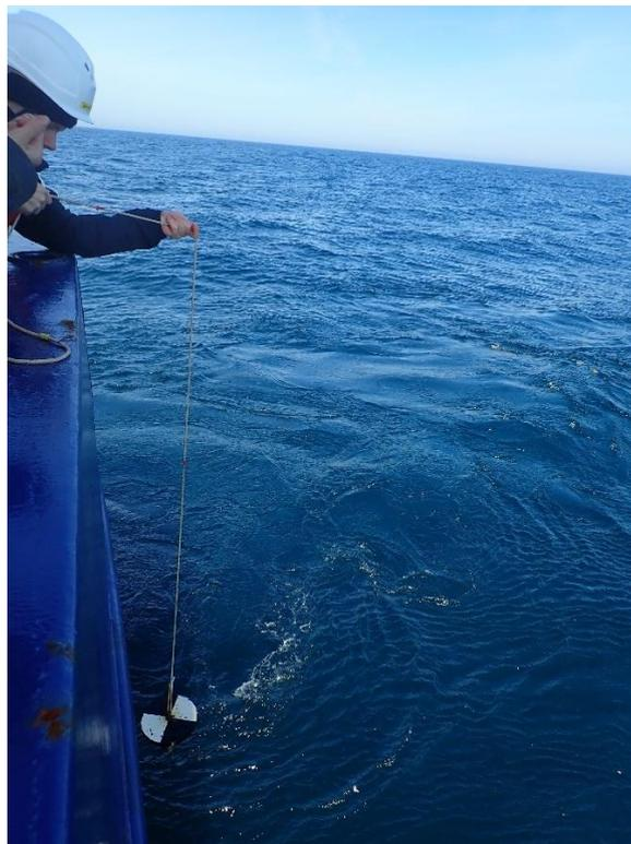
**Fig. 5.1** The SECCHI disk used during the HE639 expedition and lowering the SECCHI disk into the water.
