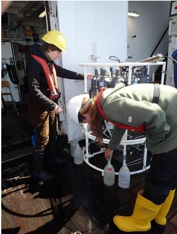
Fig. 11.7 Filling bottles with the CTD samples.
