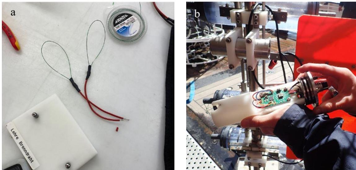
**Fig. 5.12** a) Wire loop which is used to activate the closing mechanism b) Electronic control unit
