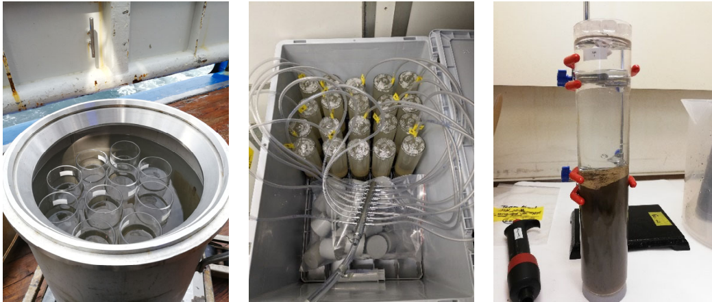
Figure 9. Perspex core liners in Box-corer (left); Cores with open caps and air supply equilibrating (middle); Sediment core before suspending it into a slurry (right).
