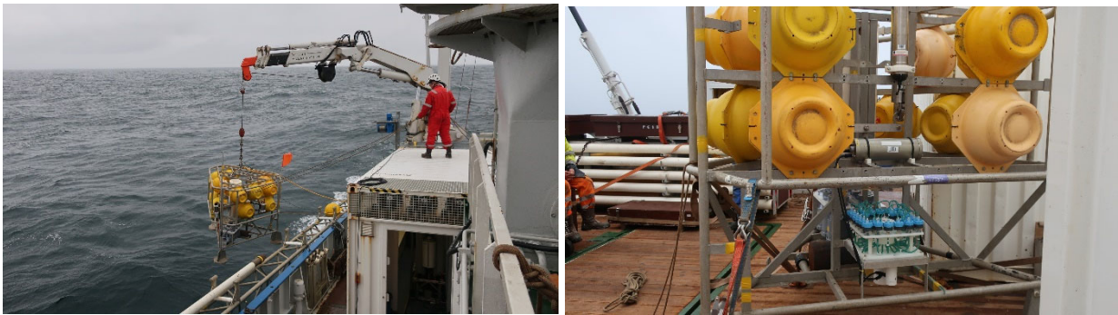
Figure 19. Deployment of the ALBEX lander (photo left). McLane pump on the ALBEX lander (photo right)
