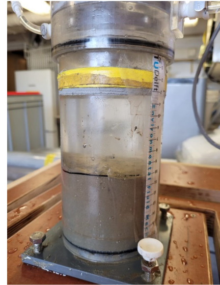
Figure 16. Gust chamber set up with sediment at the bottom and 10 cm water column.
