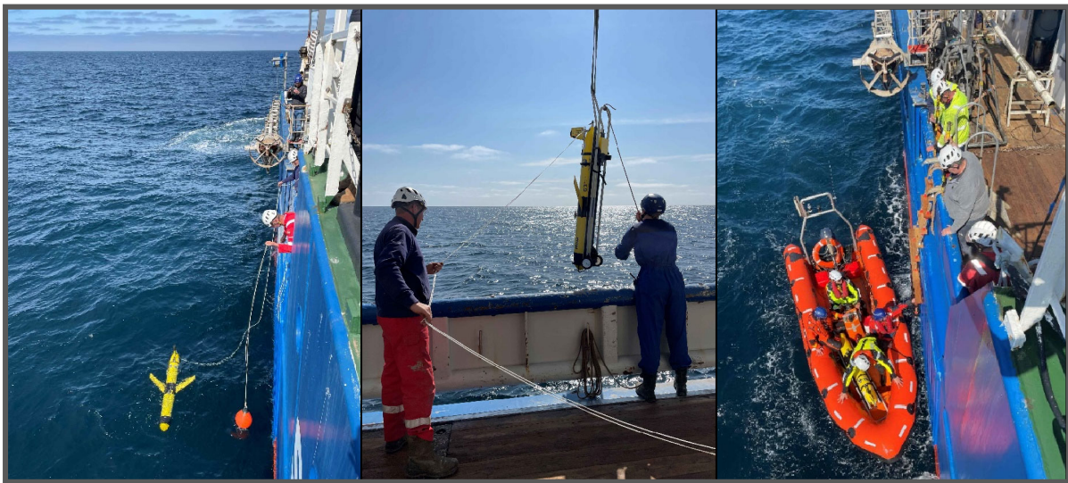
Figure 20. Photo left: Glider during preparation phase. Photo middle: glider deployment from the side winch with the auto-release module on the cart. Photo right: the glider in the man-overboard boat after recovery.
