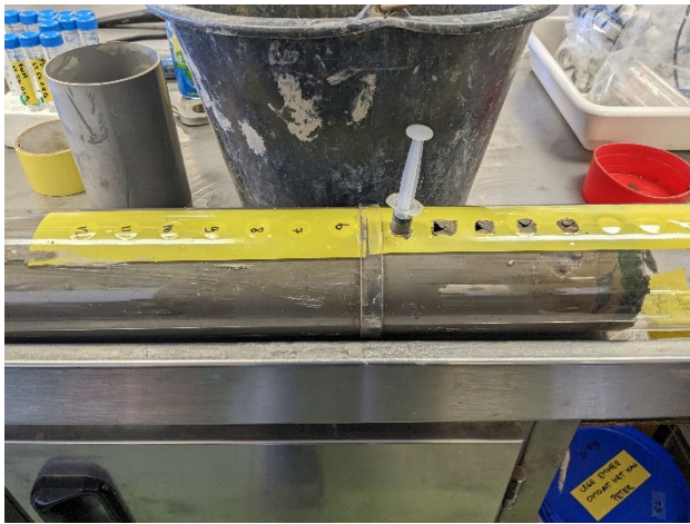
Figure 14. Stabilized core placed horizontally for sampling for 35 SO 4 experiment.
