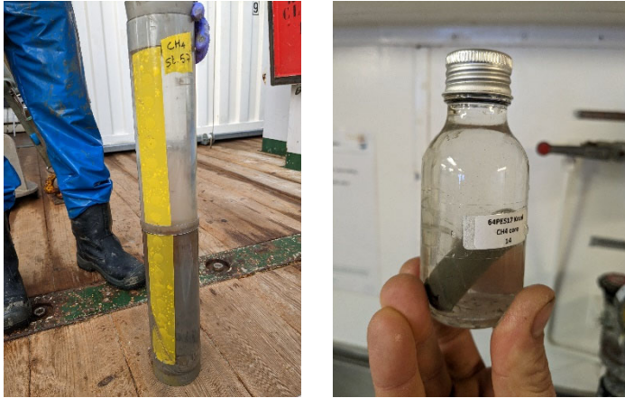
Figure 12. Core with pre-drilled holes (left); sediment sample in infusion bottle filled with NaCl (right).
