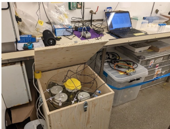
Figure 11. Set-up for whole-core incubation for benthic fluxes. Transparent tubing for sampling and water replenishment, black cables are fiber optics for O 2 monitoring.
