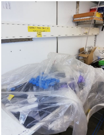
Figure 13. Glove bag with set-up for anoxic core slicing.
