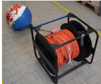
Figure 8: A picture of the custom developed drifter equipped with a logarithmic acoustic array.
