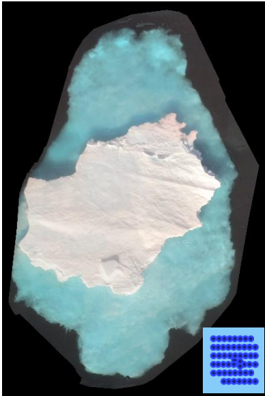
Figure 51: Orthomosaic product retrieved from the drone total track (lower right blue dots) performed on 30 th June 2023 2pm. The final size of the swath is 60 m x 40 m (lon, lat).
