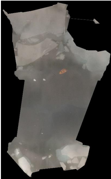
Figure 49: Orthomosaic product retrieved from the drone total track (lower right blue dots) performed on 29 th June 2023 2pm. The final size of the swath is 98 m x 61 m (lon, lat).
