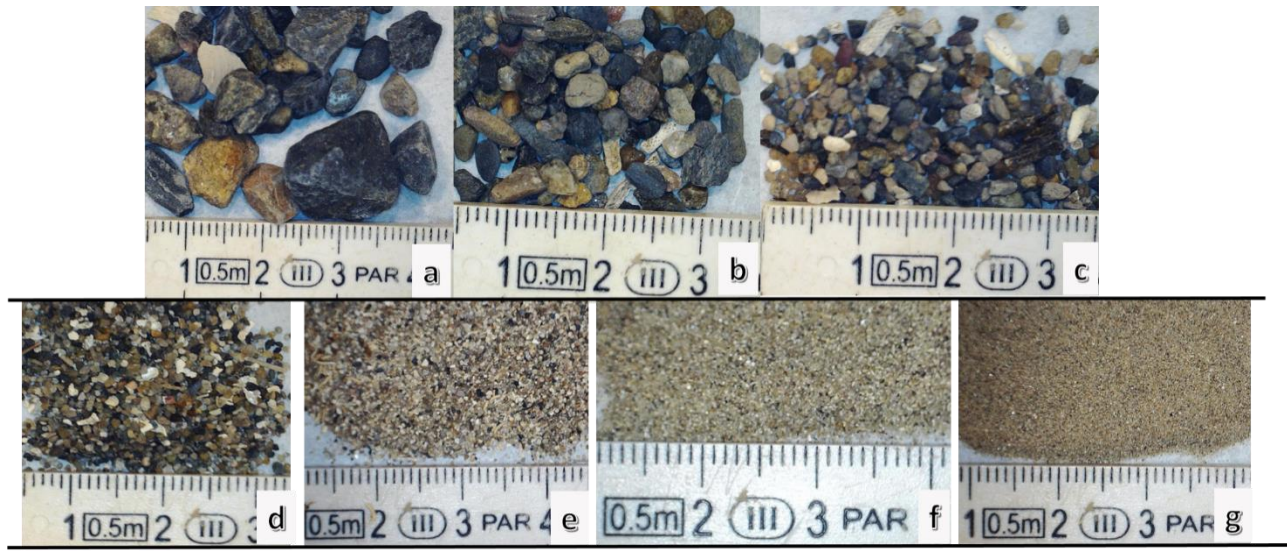
Grain size classification HN23_068_BCO_01 5-16cm
