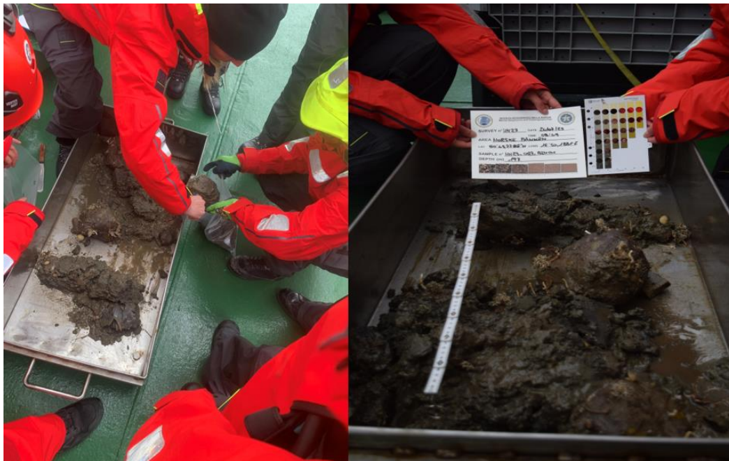
HN23 grab sampling and color determination
