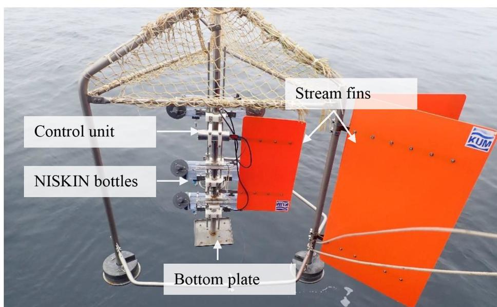
**Fig. 5.10** The bottom water sampler in use during the cruise HE619.
