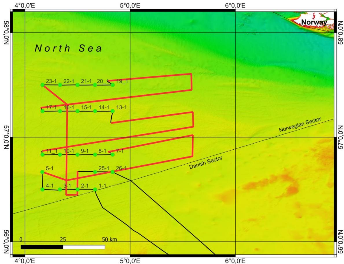
**Fig. 3.1** Track chart of RV HEINCKE Cruise HE619 with bathymetric base map. The working area is situated in the Norwegian Sector of the North Sea. Green dots indicate sampling stations with the respective number. Red lines display the hydroacoustic profile tracks.
