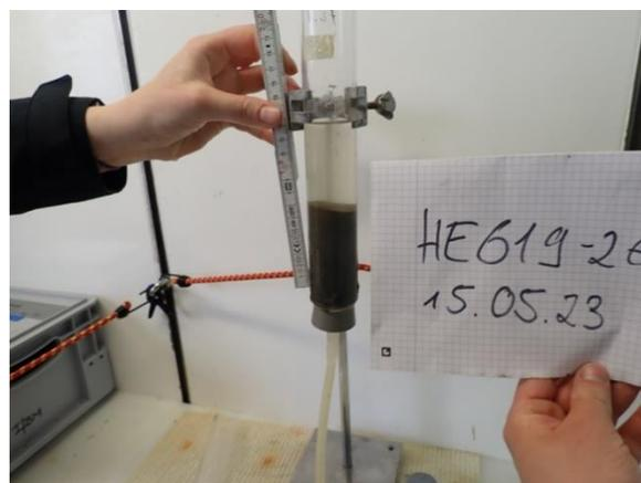
Fig. 11.4 Sediment sample from the vVG for the permeability measurement at station 26.
