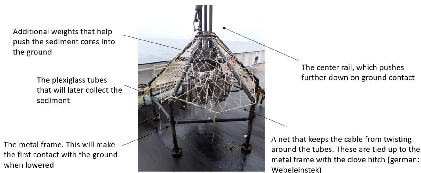
**Fig. 5.18** The Multicorer with a brief description of the components.
