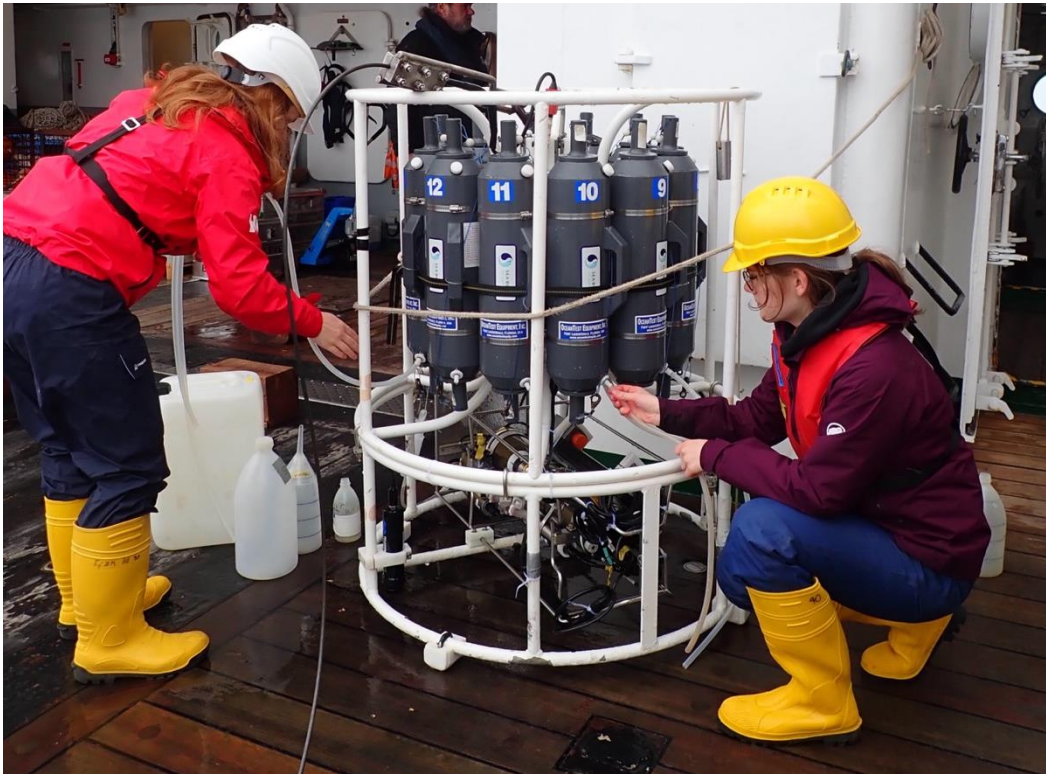
Fig. 5.6 CTD-Rosette after use in the water column. The water samples of the closed NISKIN-bottles are filled into plastic bottles for filtration.
