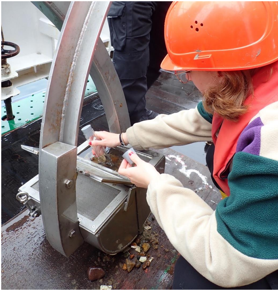
Fig. 11.11 Student taking a sample from the vVG for the permeability measurement.
