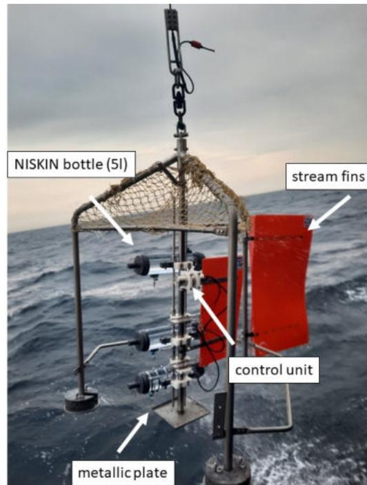
**Fig. 5.14** The BWS used in this cruise during the lifting process.
