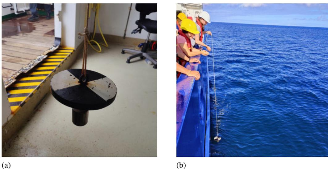
**Fig. 5.1** (a) The Secchi disc used during this cruise, (b) lowering the Secchi disc into the water.
