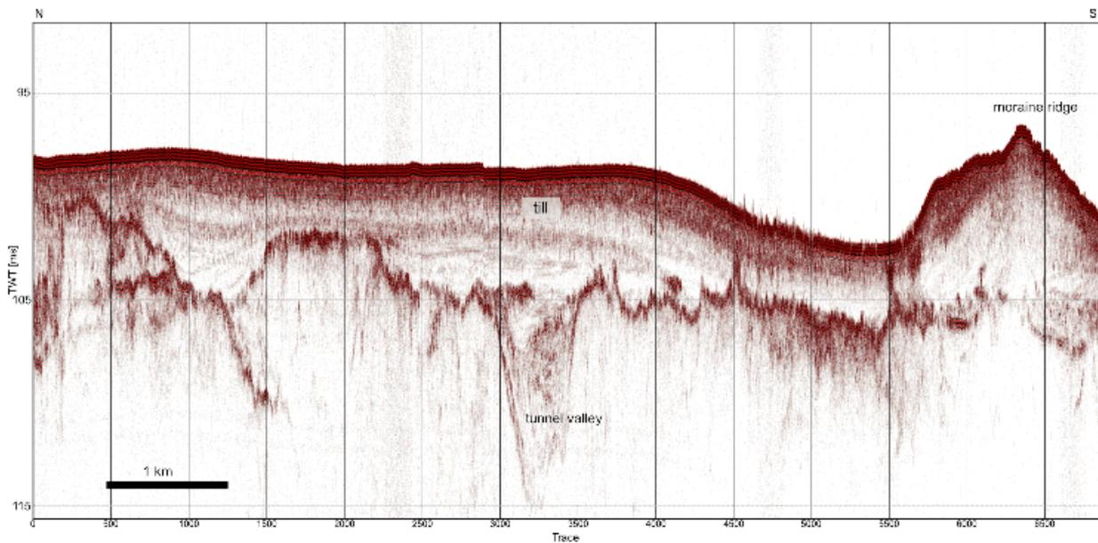
**Fig. 5.21** Second profile of the hydroacoustic survey, recorded by the sediment echo sounder SES2000 Innomar.
