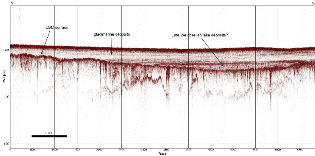
**Fig. 5.22** Third profile of the hydroacoustic survey, recorded by the sediment echo sounder SES2000 Innomar.
