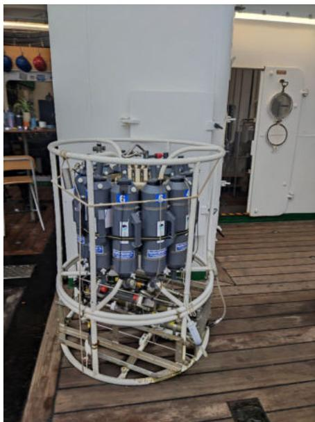
**Fig. 5.7** CTD rosette with 12 6L NISKIN bottles and the measuring instruments below.
