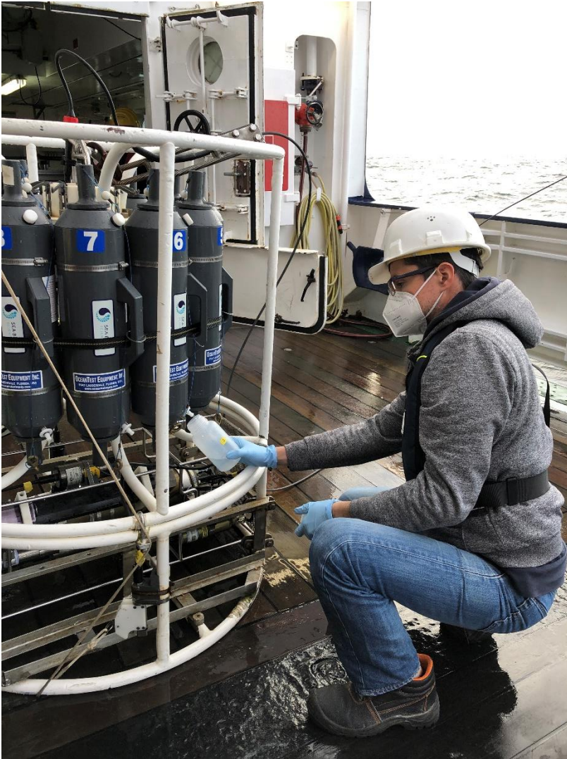
Figure 11.2.5: Taking water from the CTD (Ann-Cathrin Rohrweber / Hereon)
