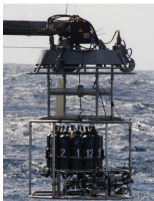
Figure 13: Picture of the lowered CTD Seabird911 system with rosette sampler and ancillary sensors ( e.g. dissolved oxygen, transmissometer, fluorometer, turbidimeter, altimeter and optics).
