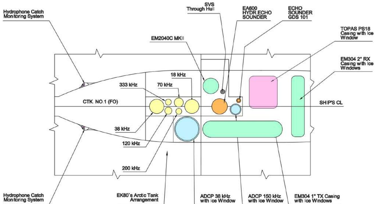
Top: Plan view of the view of the keel block where the transducers are hosted. In yellow the scientific equipment; in orange the ship echosunders.
