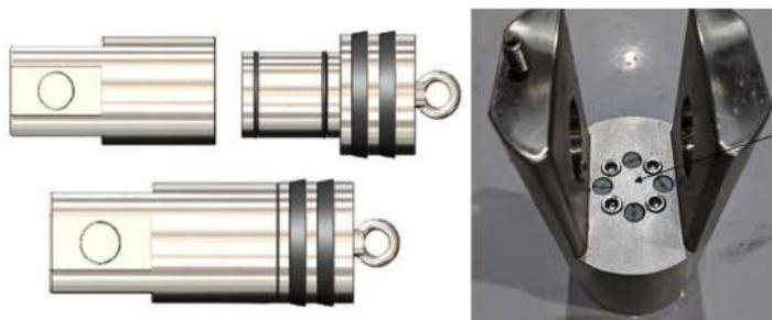
The OSIL piston is a two-section assembly which is designed to separate during operation under heavy loads (e.g. stuck piston or strong vacuum below the piston). In such cases, water flows from above the piston into a
