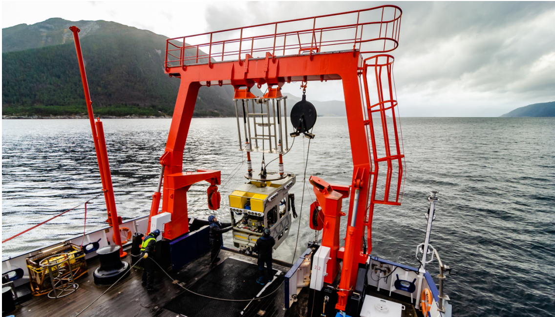
Fig. 11.1 ROV PHOCA with the LIGHTHOUSE modifications during the deployment.
