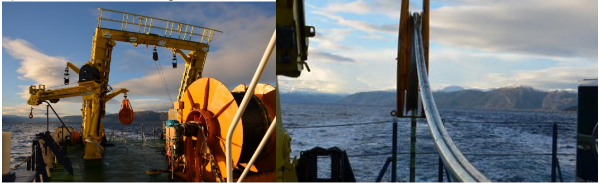
left: winch containing the towed array, right: towed array longing from the winch over the reel into the water
