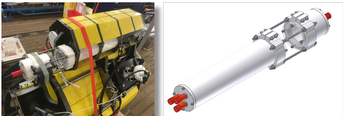
Fig. 5.3: SWIPS camera mounted on the profiler of the SWIPS winch system (left image) and a sketch of the SWIPS camera (right image)
