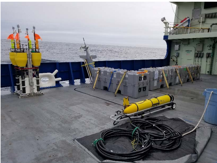
Figure 3.13: The Slocum G2 Glider Apollo, with Low Power OTA4 array, on the stern deck of the R/V Armstrong, just prior to the initial deployment on 07Sept21. The insert is a closeup of the tail, highlighting the option-added thruster, and the adaptor fitting that keeps the array away from the propellor. The drogue is shown submerged in salt water prior to the dive, and after being removed from the ship's CTD system. The drogue was sent down to 3,000m a few hours prior to deployment to eliminate extraneous air bubbles from the double braided nylon line
