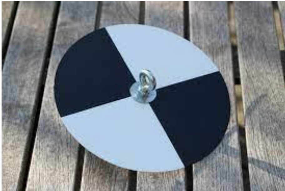
Fig. 5.1 The Secchi Disk is divided into 4 sectors (painted black and white) and is a limnological tool for a quick determination of the visibility depth in surface waters.
