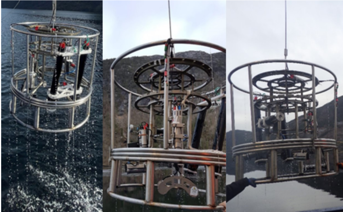
Figure 19: Three different views of the BOP, carrying CPICS, UVP5, UVP6-HF and PIScO throughout HE570.
