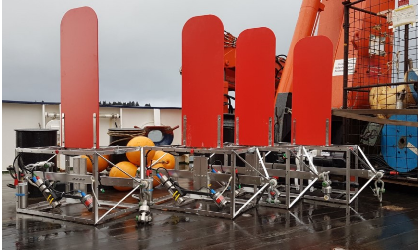
Figure 28: The four UVP6-LP mounted on their cage on the deck of FS Heincke. Two deployments were done in each of the two fjords.
