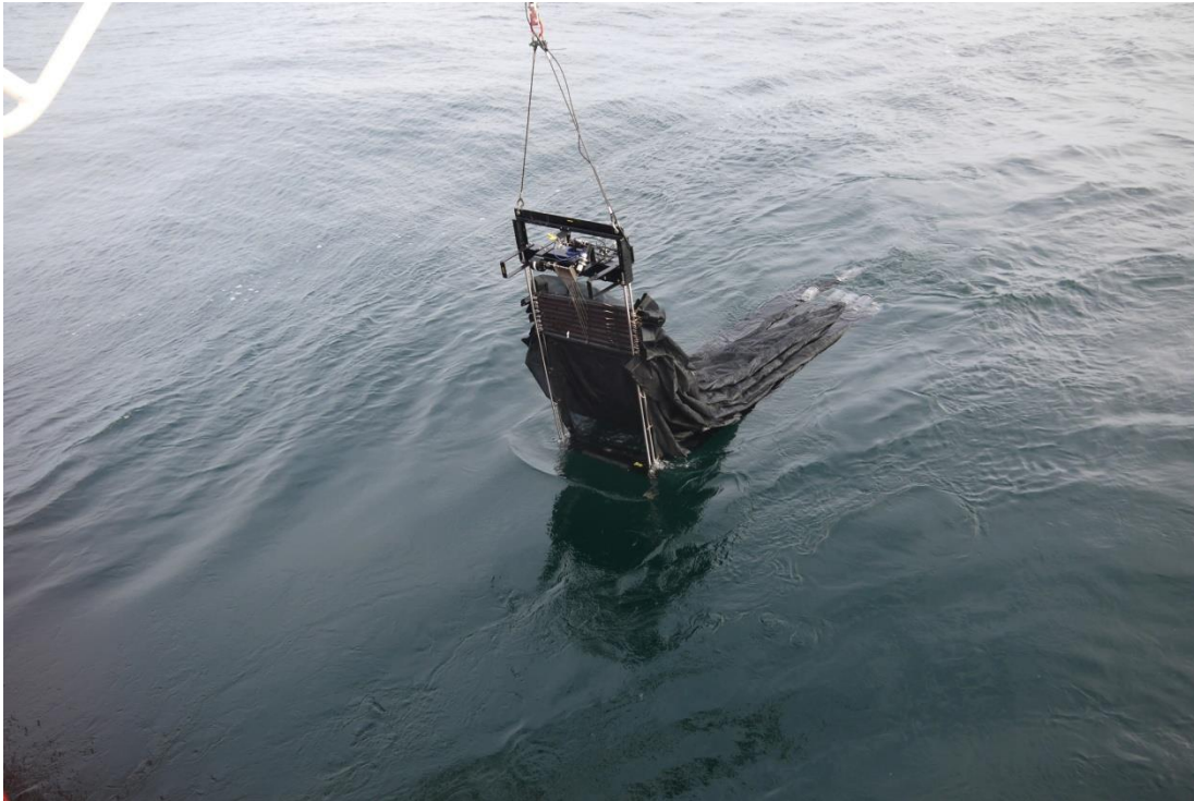
Fig 5.1: MOCNESS net at point of deployment
