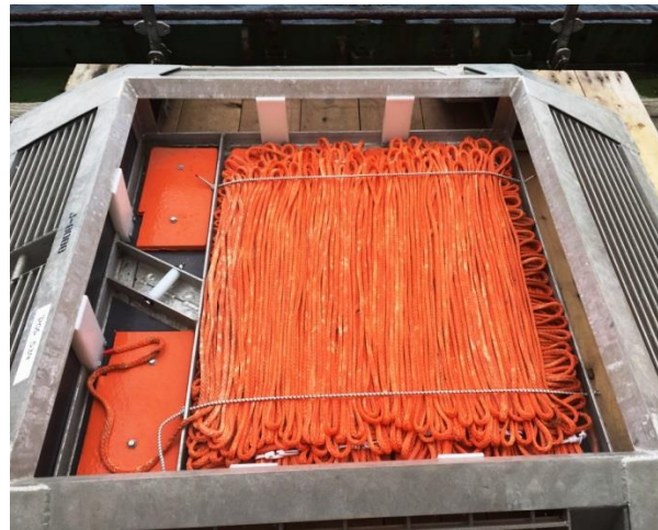
Fig. 5.7.1-2: Anchoring base with coated lead weights, Spectra line and attachment point for the releaser hook.
