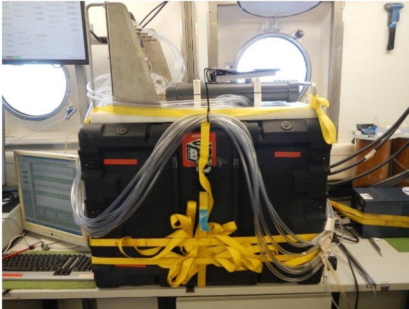
Figure 5.2-1: Atmosphere intake system (AIS) on top of black Picarro analyzer box placed in the wet lab of RV Poseidon.
