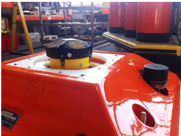
Fig. 5.7.1-3: Floatation unit with ADCP and remote releaser hydrophone mounted on top of the anchoring base.
