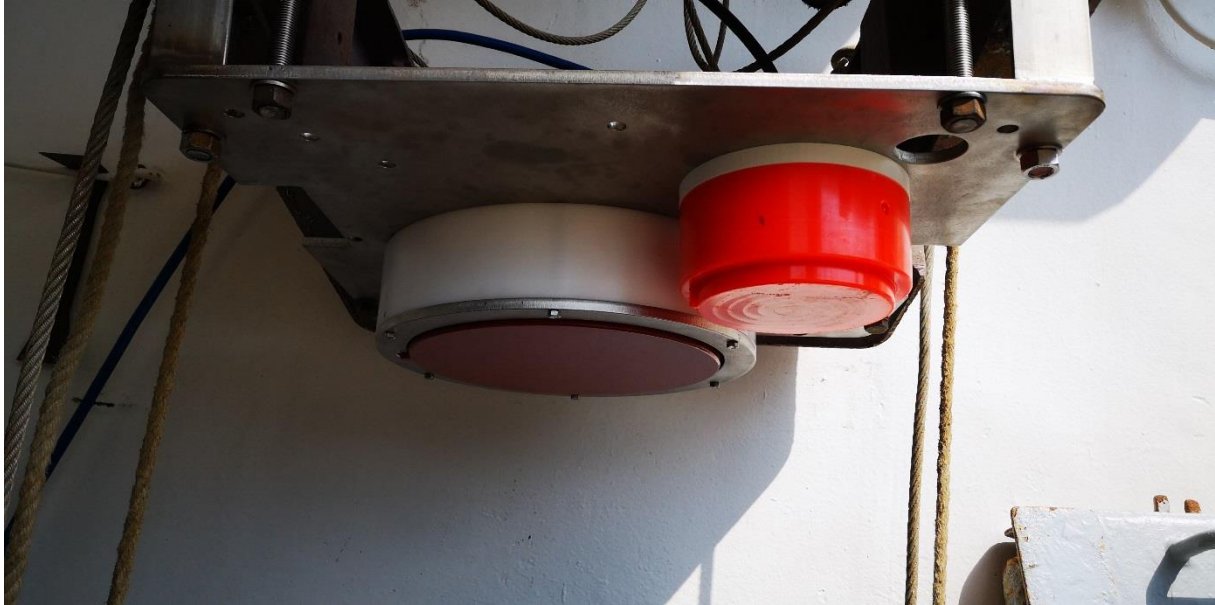
Fig. 5.1-1: EC150-3C ADCP & echosounder and ES70-18CD echosounder mounted to a stainless steel plate to be lowered into the moon pool of RV Poseidon.
