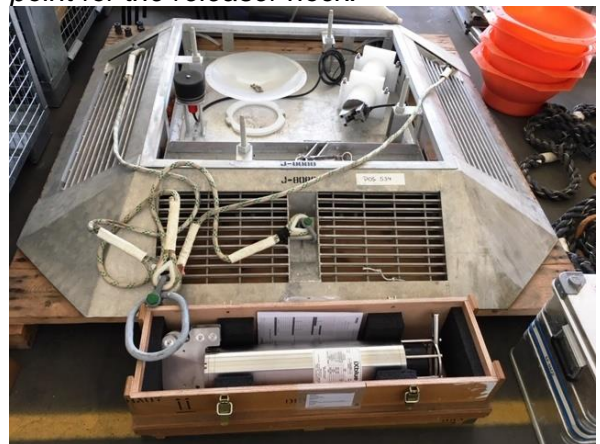
Fig. 5.7.1-4: Anchoring base with frame for the floatation unit and acoustic release with remote hydrophone placed on top of the line. In front the second acoustic releaser for deployment.
