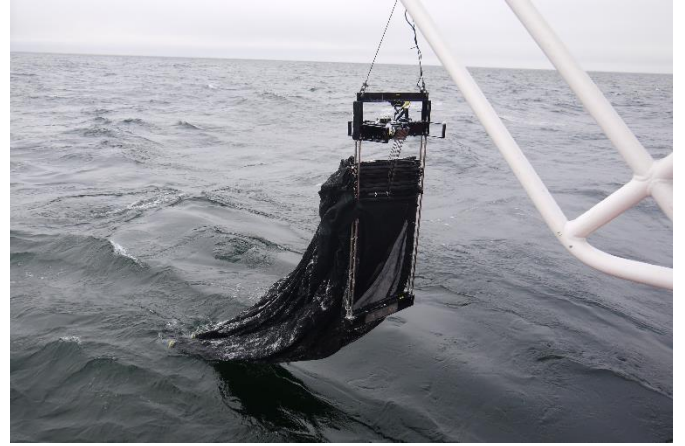
Fig. 1. MOCNESS codends being lifted over the stern ramp prior to deployment (left); MOCNESS net fully cocked at the start of a deployment (right)
