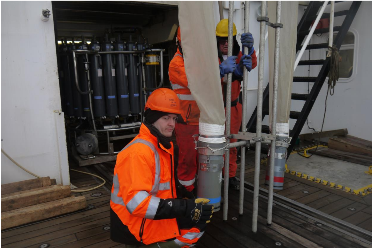
Fig. 1 Cod-end buckets being clasped on prior to deployment
