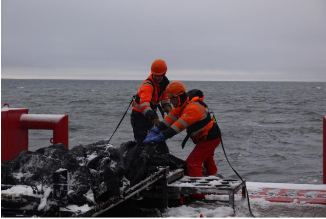
Fig. 1. MOCNESS codends being lifted over the stern ramp prior to deployment (left); MOCNESS net fully cocked at the start of a deployment (right)
