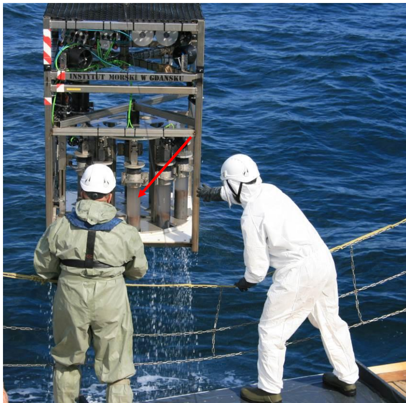
Figure 6 Multi-increment revolving sampler constructed at Maritime Institute Gdańsk. The sampler allows ten single sediment samples (red arrow) to be collected from the sea floor in one dive. (Photo: FFI)
