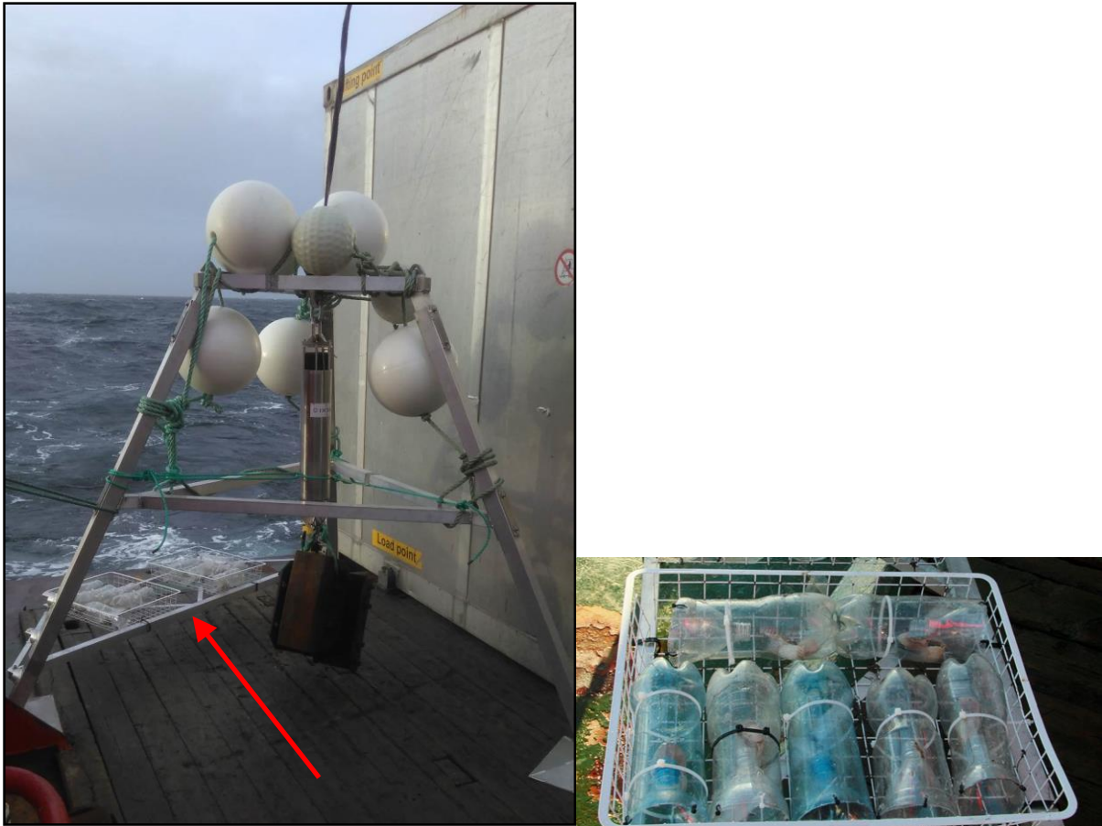
Figure 7 Rig with hagfish traps (red arrow) and soda bottles with fish used as bait. (Photo: FFI)
