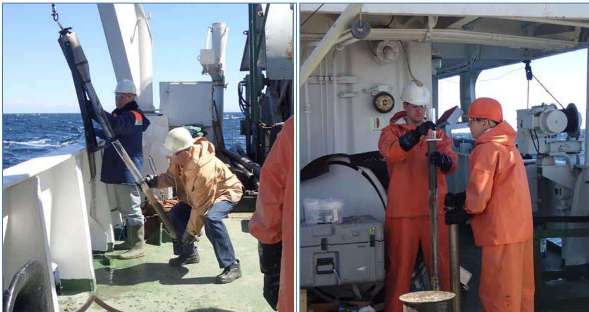
Figure 5 Sampling work on-board Akademik Strakhov in the Måseskär area in June 2017. A Niemesto corer from SIO was used to take virtually undisturbed sediment samples. These were later processed for Arsenic (analysed at CTH), for degradation products of chemical weapons (analysed at VERIFIN) and for meiofauna (analysed at IOPAN, Poland). (Picture from [10])
