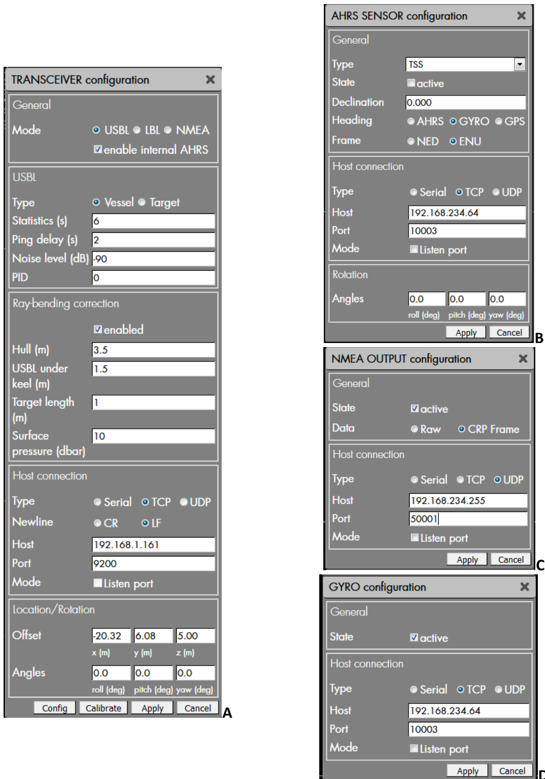
Figure 87: A: Transceiver configuration sets the main parameters of the system. Mode enables the internal AHRS; the Host connections links the SiNAPS software to the modem; the USBL settings gives the frequency of the pinging between the USBL system and the beacon on the AUV/JAGO (here 2 seconds). B: AHRS here means external motion sensor input. This was not used (State is not checked) and thus the internal motion sensor was used (see image A). C: Output was given to OFOP and others via a UDP port. Using the IP address of xxx.xxx.xxx.255 means that all PCs in the respective subnetwork (234) can receive the messages (here PTSAG data) when listening on port 50001. D: Heading of the ship was used as input (State = active), in this case it came via a TCP connection on port 10003, alternatively it could come from separate sensor (Octans, or similar) but could also come from the AHRS of the Evelogics system.
