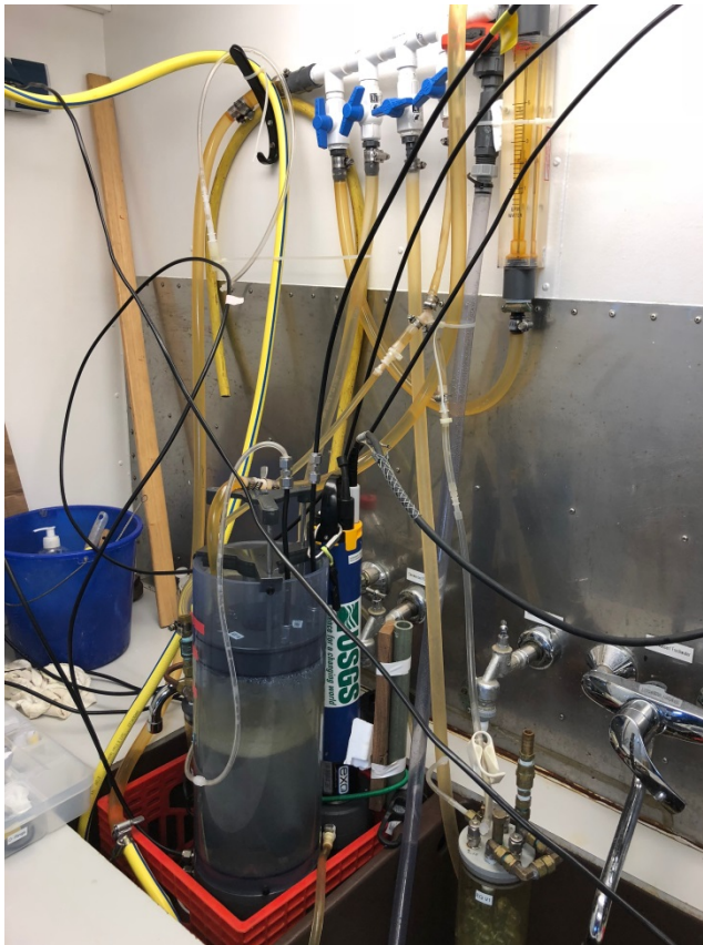
Figure 18: YSI Exo2 datasonde and Weiss Equilibrator system on board of RV POSEIDON.
