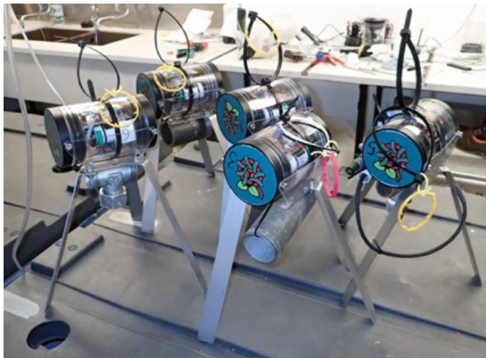
Figure 29: 5 PiCams mounted on deployment tripods, with additional 1 kg weight added.
