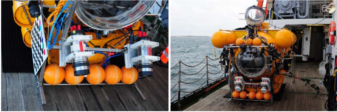
Figure 27: The two pressure housings with flat optical port mounted to JAGO. Left: JAGO also carries a chessboard for underwater camera calibration.
