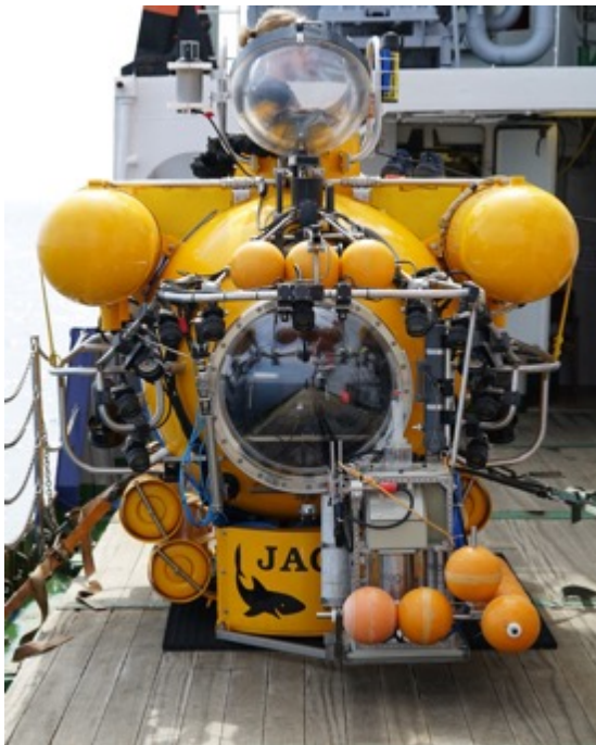
Figure 21: Bubble box as attached to the front of JAGO.
