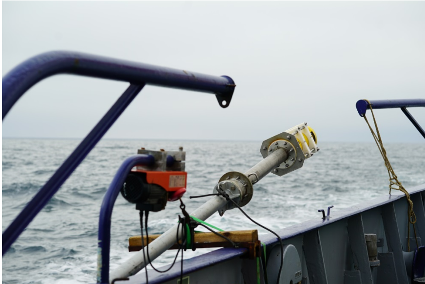
Figure 36: ADCP installed on the starboard side pole of RV POSEIDON.
