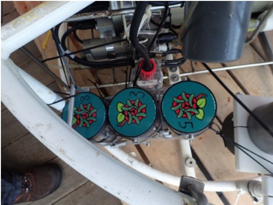
Figure 31: Array of 3 PiCams mounted on the TV-CTD, adjacent to the main camera.
