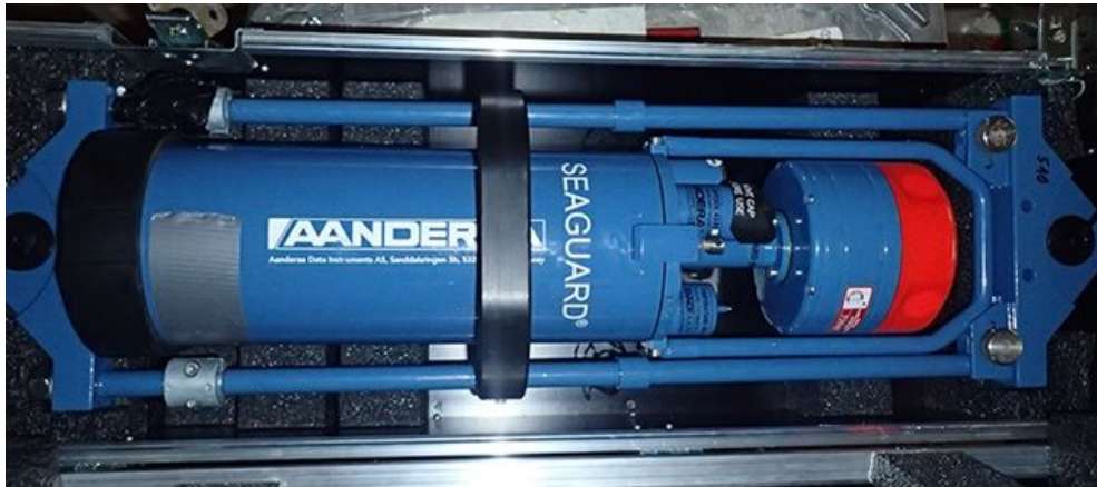
Figure 33: AANDERAA Seaguard RCM deployed at station POS526_95_TV-CTD_57 to POS526_99_TV-CTD_61.
