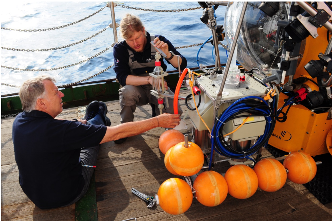
Figure 8: BubbleBox and gas sampler installed on JAGO.
