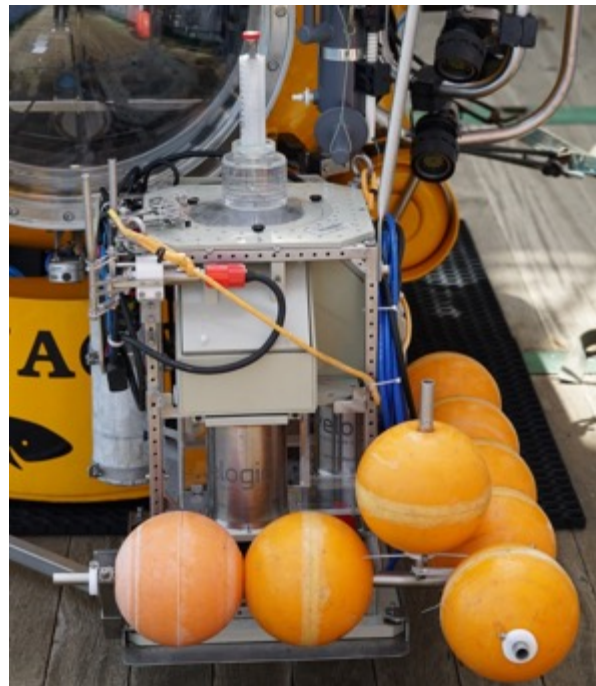
Figure 21: Bubble box as attached to the front of JAGO.
