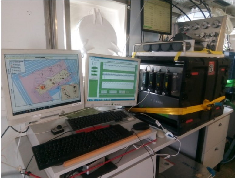
Figure 13: OFOP PC, Picarro and Atmosphere Intake System in the Wet Lab (left); air inlet on the top deck (right)
