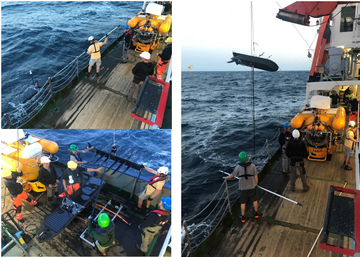
Figure 12: WaveGlider recovery at the Dogger Bank working area.
