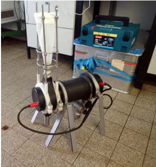
Figure 32: The LOKI ROV camera, configured for desktop use during POS526.
