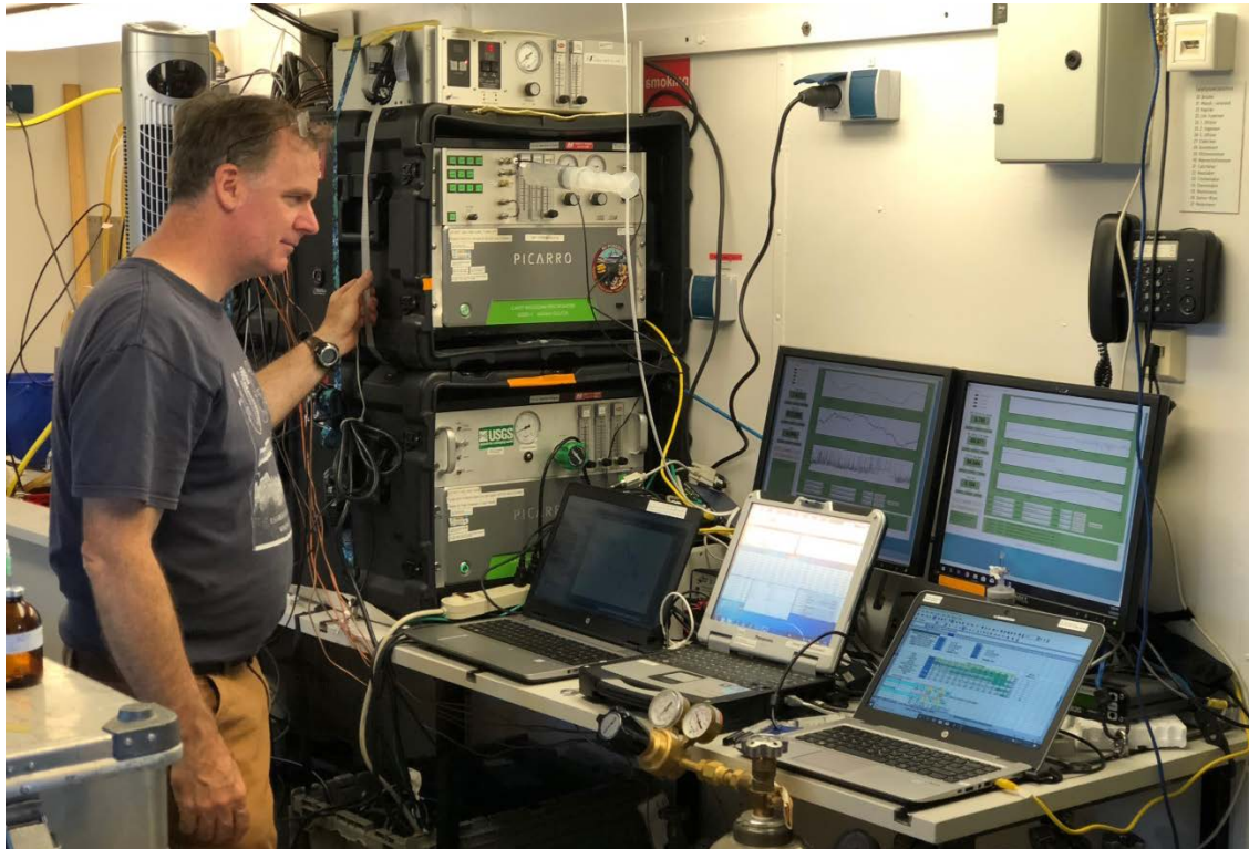
Figure 16: USGS AGS and DSAM system, the top Picarro unit is the DSAM system with a large syringe for injection of the gas sample.
