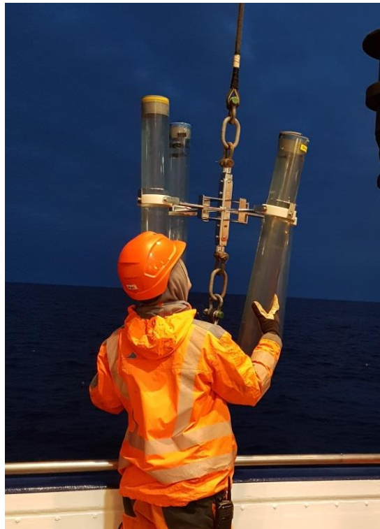
Fig. 5.3.1 Free-drifting sediment trap during deployment with one of the trap stations with the four trap cylinders.
