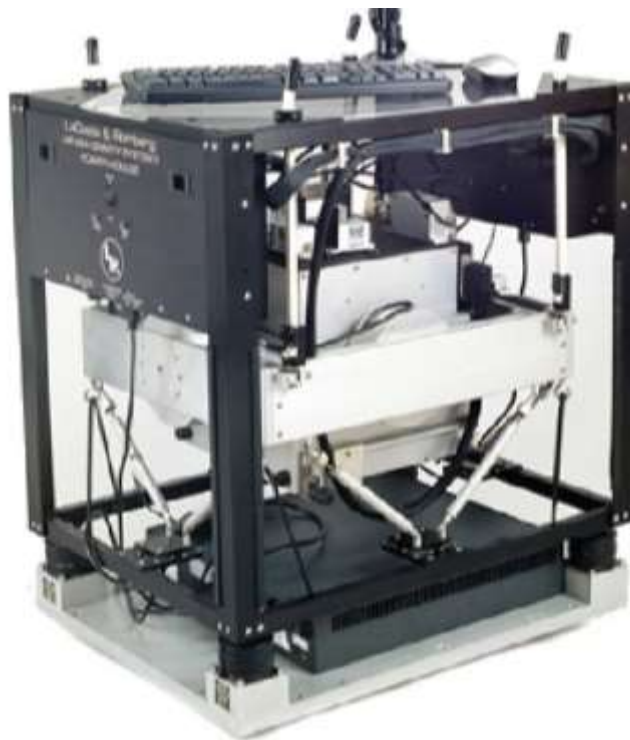
Figure 46– Example of a gravity meter for onboard installation
