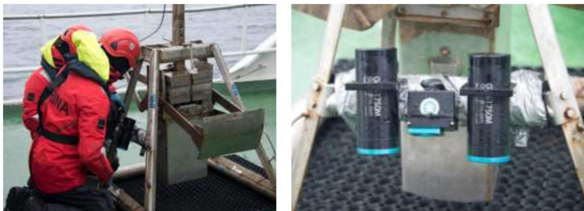
Figure 27. Box-corer used in High North 18 with the GoPro camera and two spotlights placed on a side of the box-corer.
