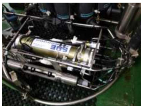
Figure 3 Water sampler device (Rosette) equipped with 12 Niskin bottles (5L capacity) and CTD probe. The table on the right reports the configuration of the CTD 9 11plus used during HN18 cruise.
