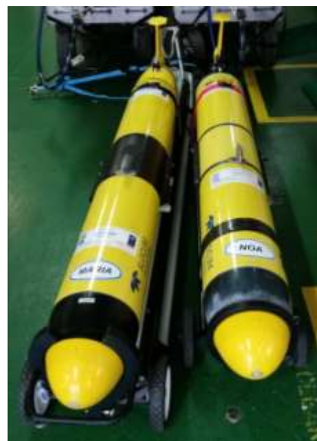
Figure 14. Gliders Maria (right) and Noa (left). The larger size of Maria (G2 with extended batteries) compared to Noa (G1 with standard batteries) can be noted.
