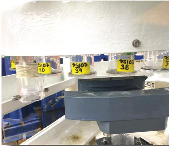
Fig 4.6: The old BOP system deployed during PS107 and recovered during PS114 with the glass settling column and camera system (a: left image) and the rotation table with collection cups (b: right image)
