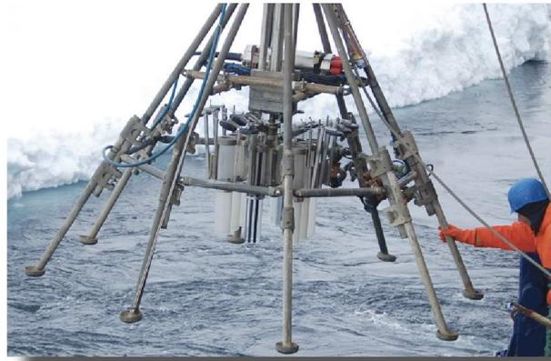
Fig. 4.3: Sediment sampling using a video-guided multicorer (TV-MUC)
