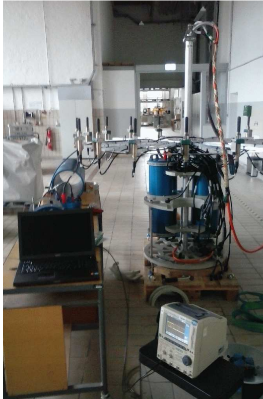
Figure 2: Drifting circular hydrophone array with 18 hydrophones.
