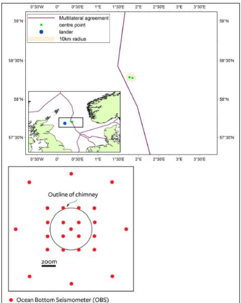
Figure 2: Schematic illustration of possible layout of seabed instruments within survey area. Surve lines will extend outside this central area.
