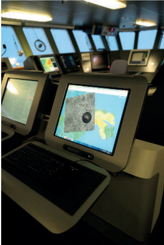
Fig. 10.4: Bridge computer with viewer for data visualization during operation: Here, an up-to-date (3 hours old) Sentinel-1 radar image is displayed together with data from the ship radar and a bathymetric chart.
