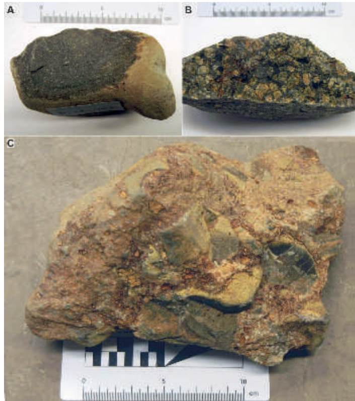
Fig. 4.6: Recovery from station PS101/193-1 at the northwestern Karasik slope. A: Fine grained basalt (PS101/193-R1); B: basaltic rock with large phenocrysts of olivine and plagioclase (PS101/193-R3); C: brecciated rock with volcanic rock clasts (PS101/193-R5).
