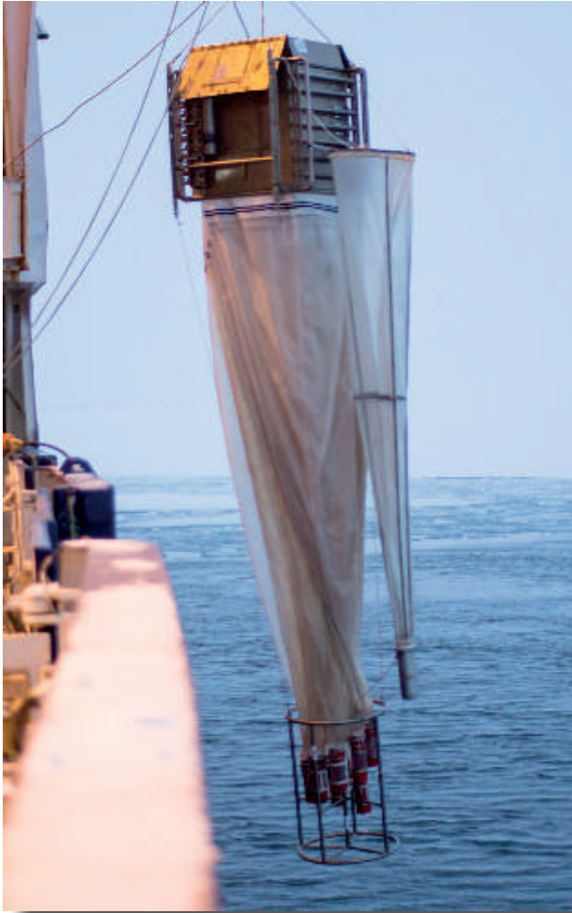
Fig. 7.1: The Multinet Maxi with the attached side net. Picture: Frederick Tardeck (FIELAX)
