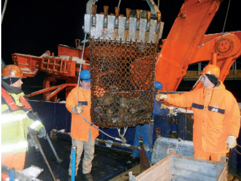
Fig. 4.1: Chain bag dredge back on board after successful deployment at the Vent Site
