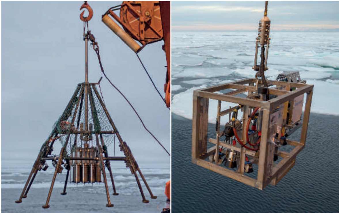
Fig. 3.4.1: Vehicles for habitat mapping: OFOS (right) and TV MUC (left) (F. Tardek, S. Dreutter)
