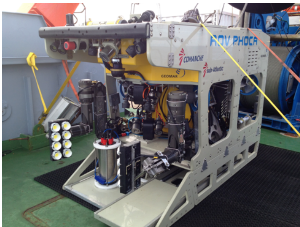
Figure 8.1 ROV Phoca with the DeepSurveyCam mounted on the front porch.
