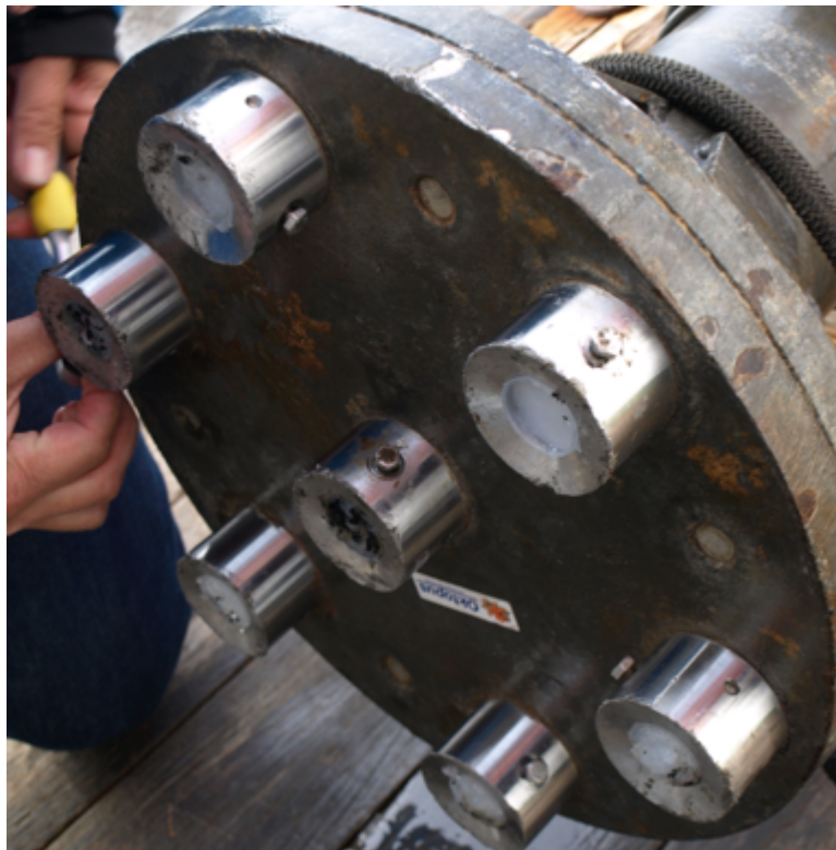
Fig. 7.2: The head after a successful deployment showing glass chips caught in the wax filled cups
