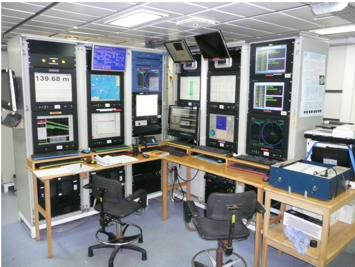
Figure 7. Geophysical and hydrographic corner of the main lab. All scientific equipment including multibeam, sub-bottom profiler, navigation systems, Olex, USBL are rack mounted.
