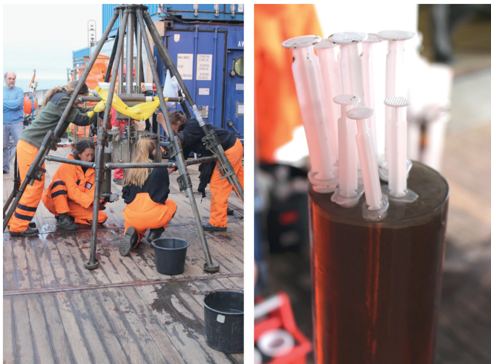
Fig. 3.4.1: Retrieval of surface sediments using a multiple corer (left); Subsampling of multiple corer tubes with plastic syringes (right)
