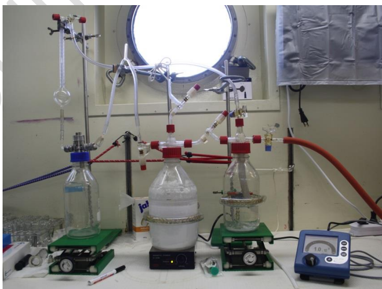
Fig. 20: Setup of the vacuum extraction on the cruise.
