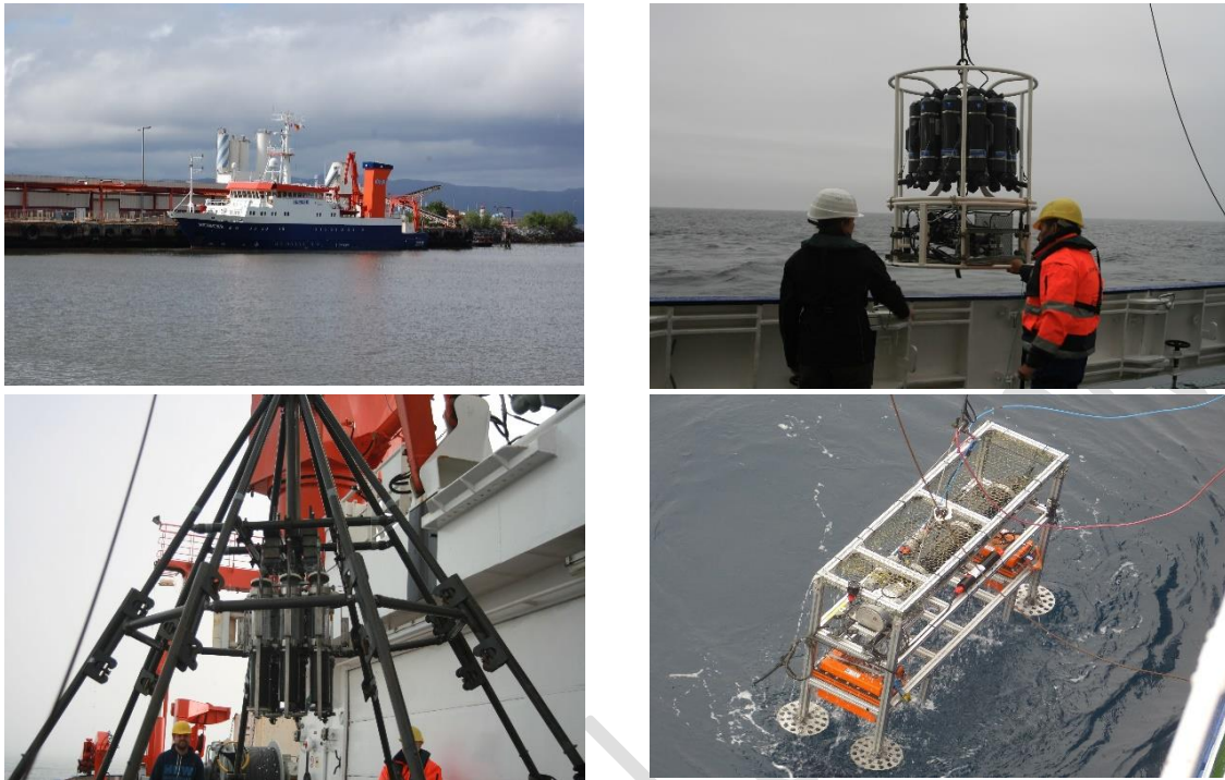
Fig. 2: Research tools used during cruise HE449. R/V HEINCKE in the port of Trondheim, Norway (above left); CTD-water sampler on the working deck during the launching (above right); conventional multi-corer comes back from the seafloor (below left) and the underwater mass-spectrometer (UWMS) deployed from the vessel (below right).
