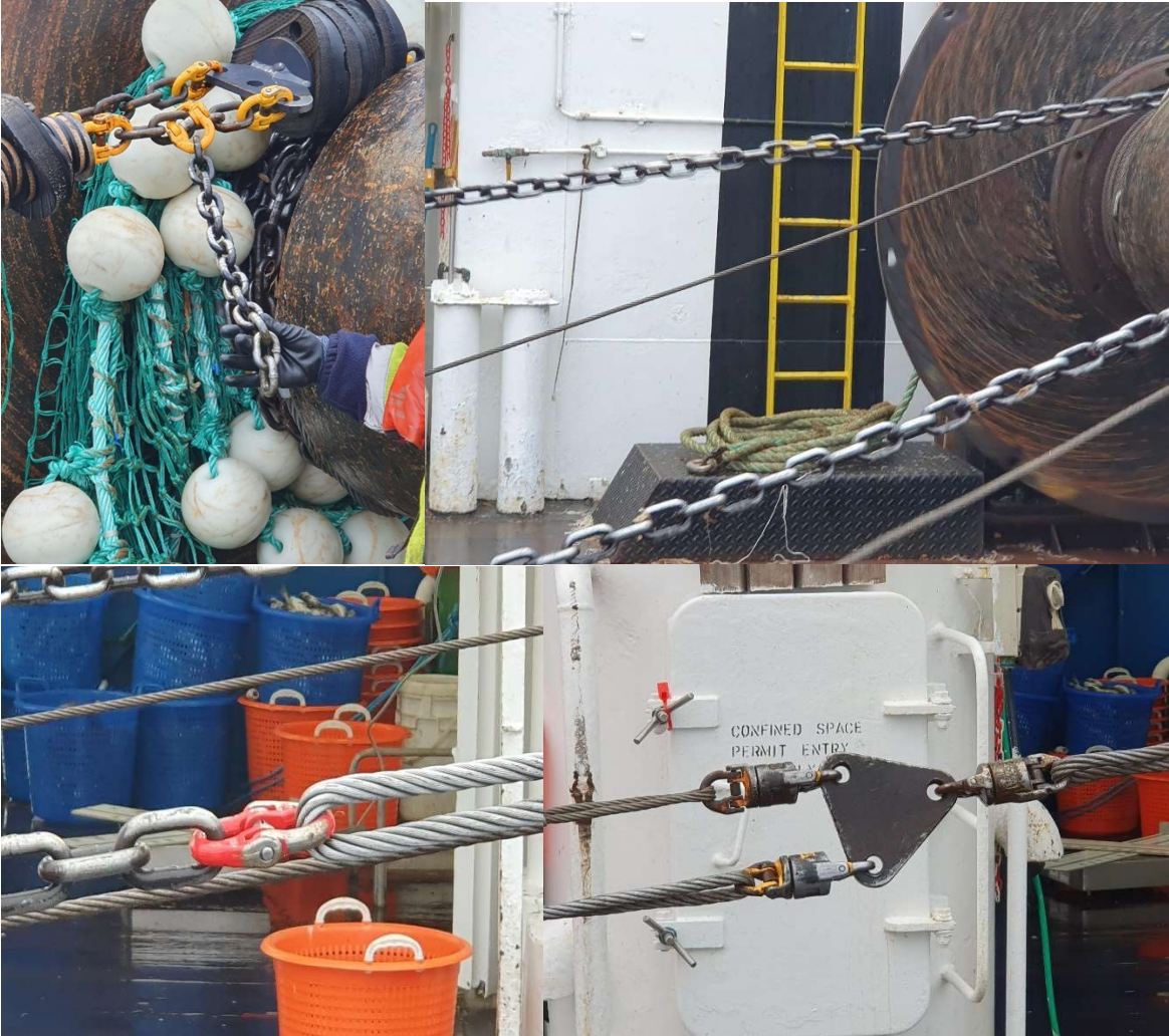
Figure 5: abrasion on dangle chain, ground extension chain, hammerlock between sweep and extension chain, and triangle split
