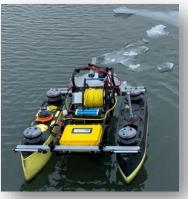
Study area with stations marked by red dots. The sampling by bathometer rosette with CTD and surface remotely operated vehicle
