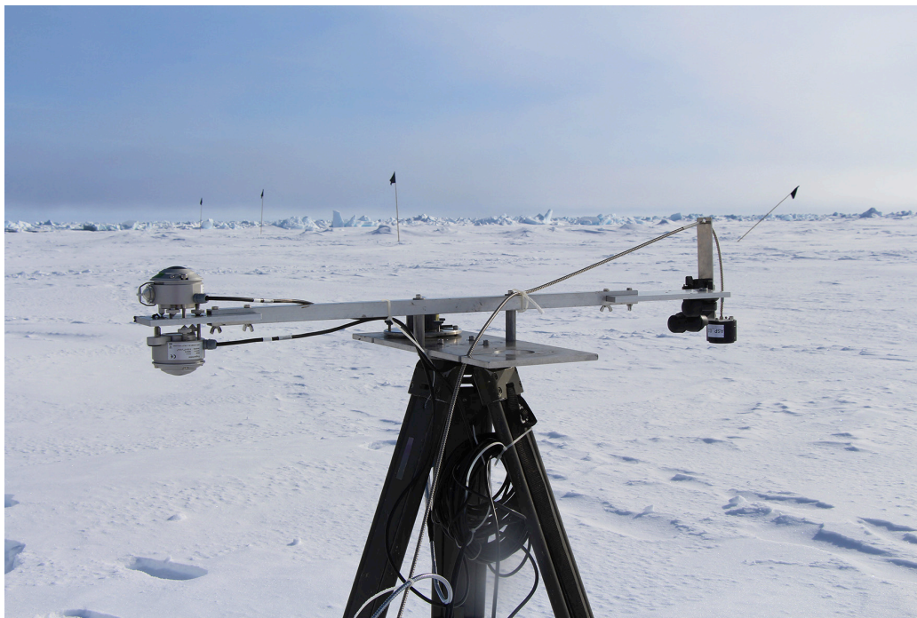
Fig. 3.4: Tripod from CORAS with broadband pyrgometers (left) and spectral irradiance inlets (right) on the ice floe during PASCAL
