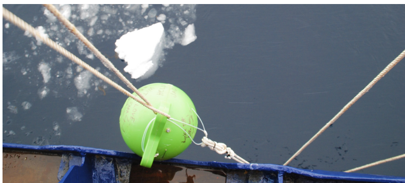
Fig. 9.6: Deployment of LoTUS 41 by lowering with two ropes
