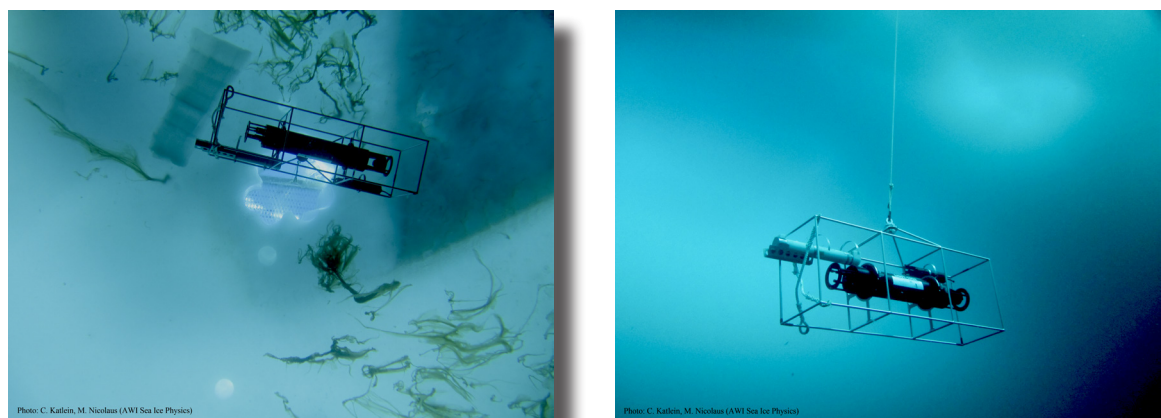
Fig. 9.4: Photos of the LISST taken by the ROV team during the overnight deployment just below the sea ice (3 m depth) (left) and the 48-hr deployment at 25 metres depth (right). The LISST is the larger instrument in the centre of the frame, while the smaller white instrument is a MicroCAT CTD, and the smallest black instrument is an AQUALogger for turbidity. )
