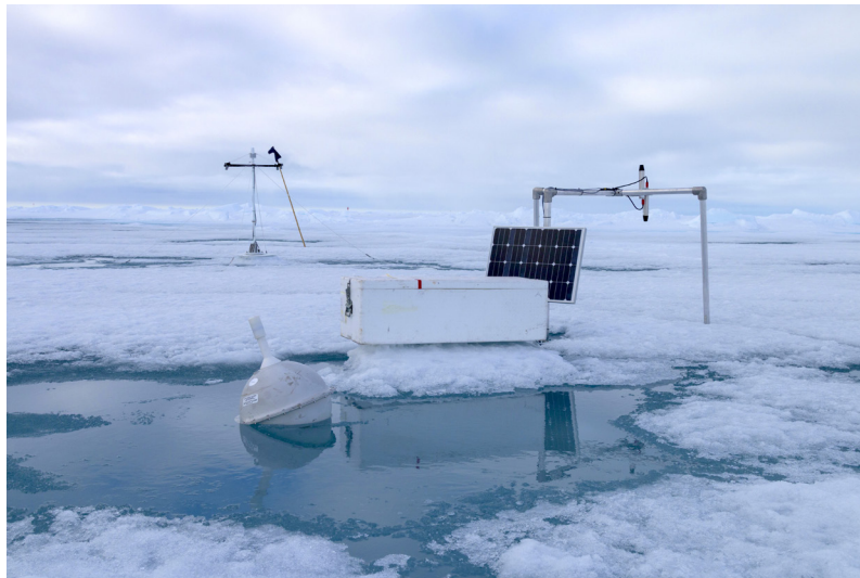
Fig. 10.6: The buoy station before recovery on 12 July. Only the surface velocity profiler (see Fig. 10.5b) remained on the ice to enable the continued tracking of the floe.
