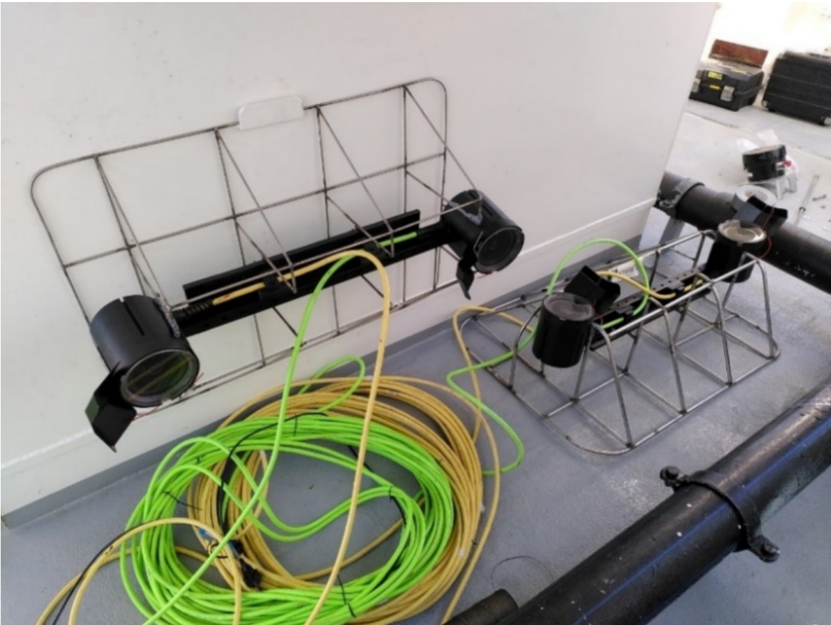
Figure 7: Stereo camera systems rigged prior to deployment on the side panels of the transfer channel.
